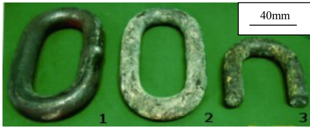
Fig.1 Chain links of 105NA (1.4892) steel: 1 – a new before mounting, 2 – link in operation, 3 – link destroyed after operation.
